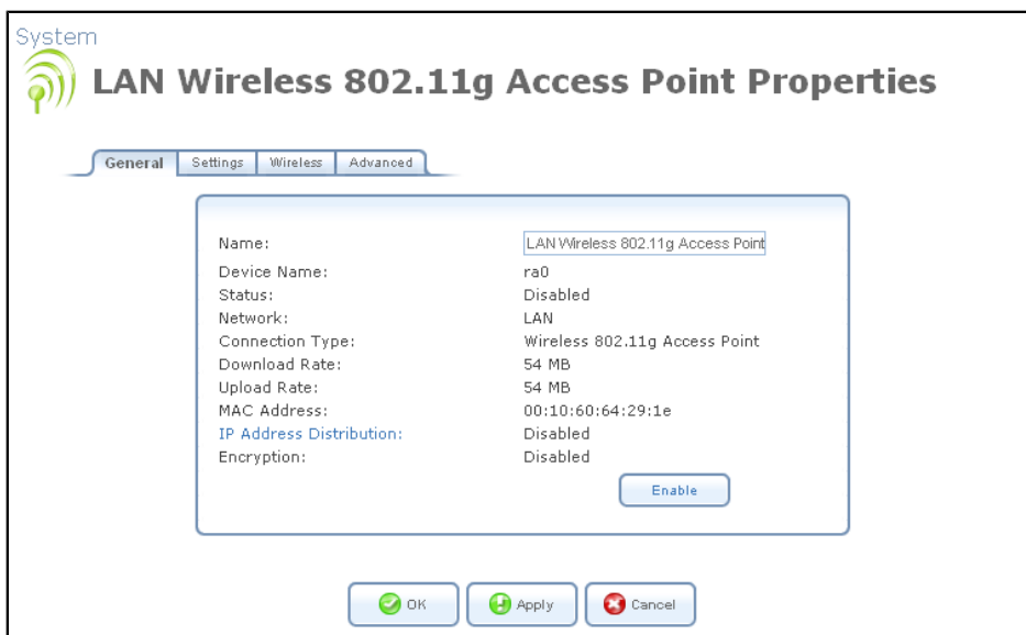
Figure 8.64. LAN Wireless 802.11g Access Point Properties – Disabled
