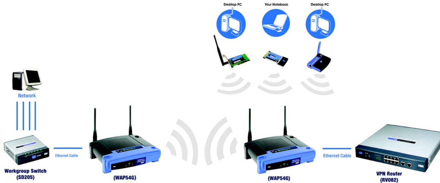
Figure 6-6: Wireless Repeater Diagram
