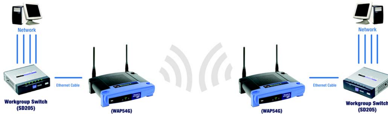
Figure 6-7: Wireless Bridge Diagram
